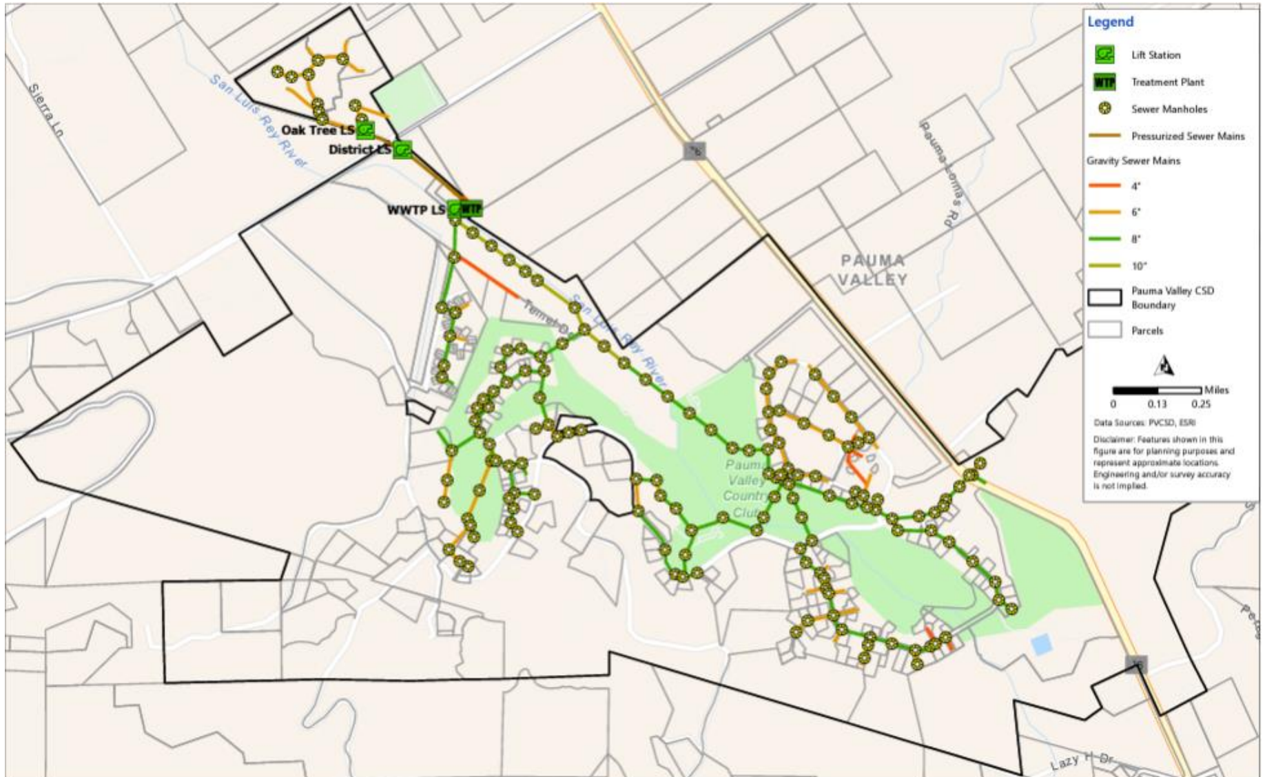
Figure 1 Sewer System Overview
